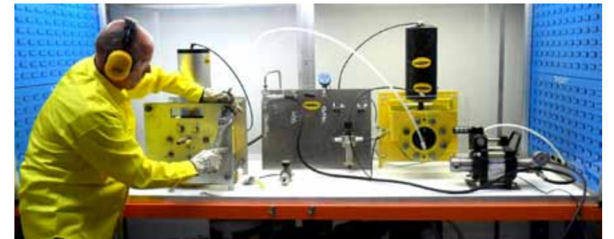
Pressure testing sleeves under controlled conditions
