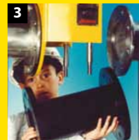
3 Remove worn sleeve and replace with new sleeve
