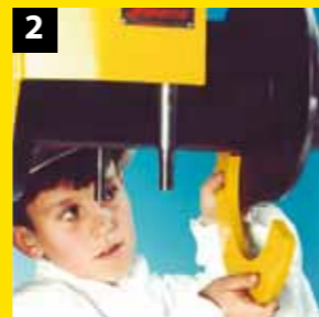
2 Remove flange bolts and backing flanges
