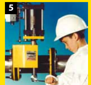
5 Replace lower pinch bar and tie rod pins
